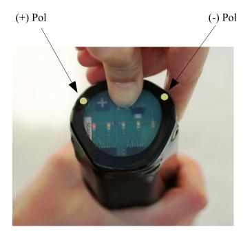
image shows the battery has a 80% state of charge
