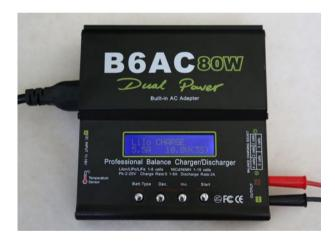
Set the desired charging current. The battery for a maximum charging current of 10A is approved. However, we strongly recommend a charging current of 5A – 6A.
